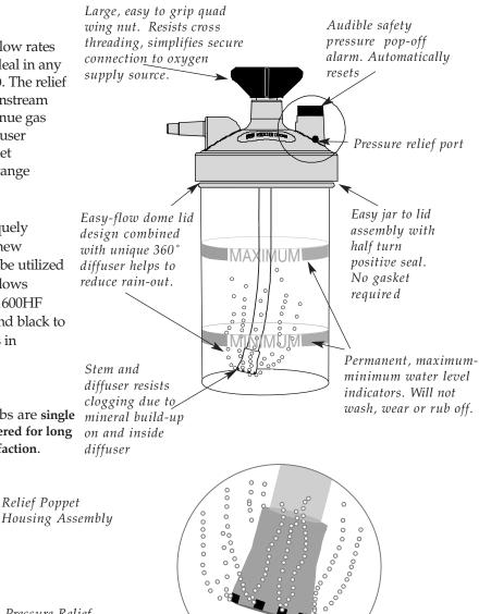
Unique 360° rectangular diffusion ports operate quietly with improved hydration and less system back pressure.
